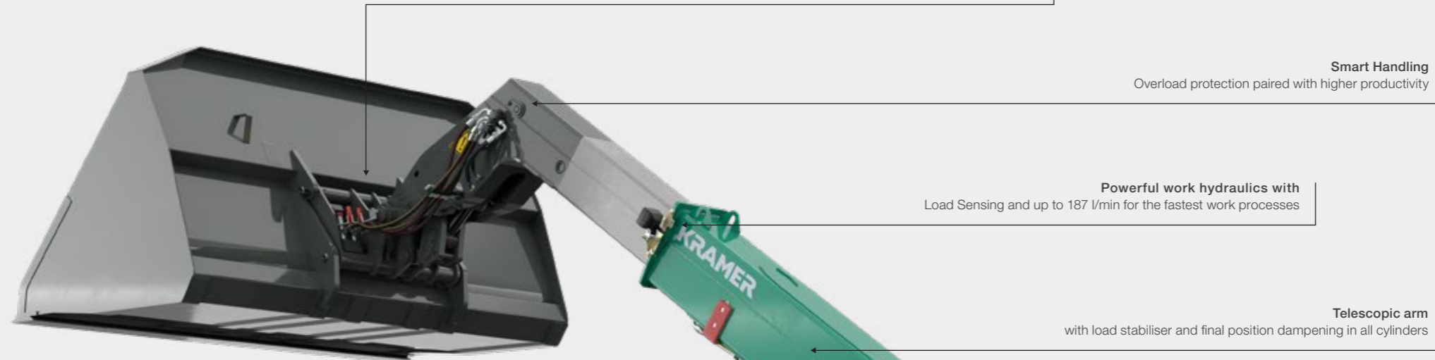
Solid quickhitch plate with four connection points (each 50 mm diameter) for the perfect seat of the attachment
