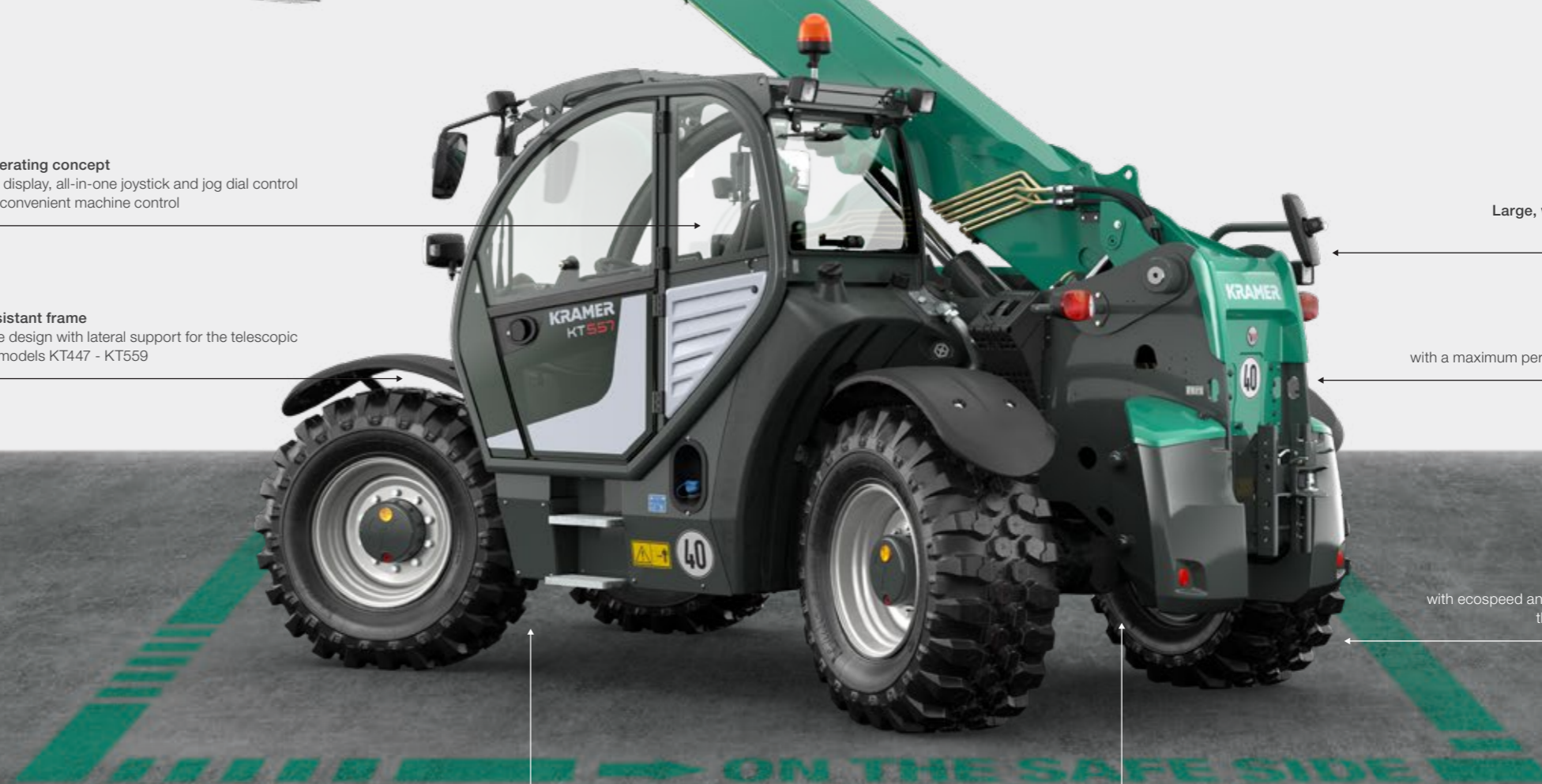
Telescopic arm with load stabiliser and final position dampening in all cylinders
