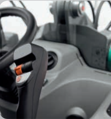
Sensitive and precise control of the machine and attachment via mechanically, pilot-operated joystick.
