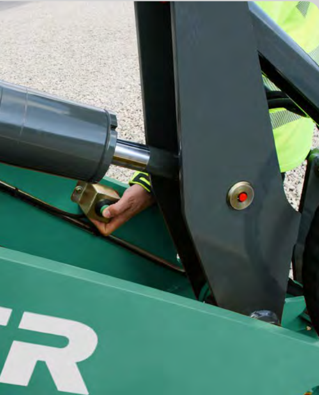
Pressure release in the 3rd control circuit – for easy connecting and disconnecting of attachments with hydraulically activated auxiliary functions.
